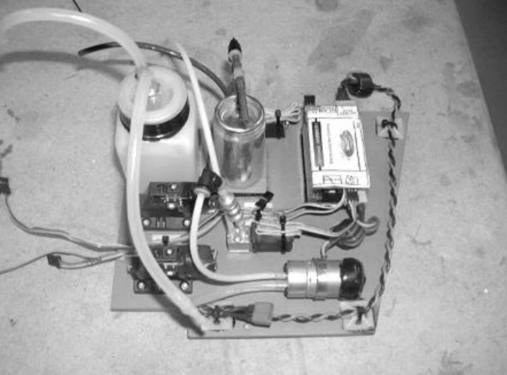
Suggestion for a removable equipment plate that fits in front of the main tank.
