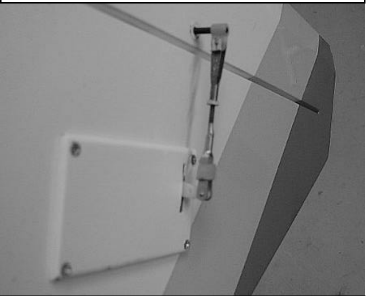
RUDDER CONTROL ROD
